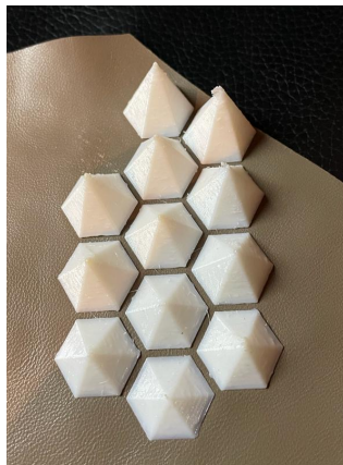
Top view on 3D printing on leather with PLA
