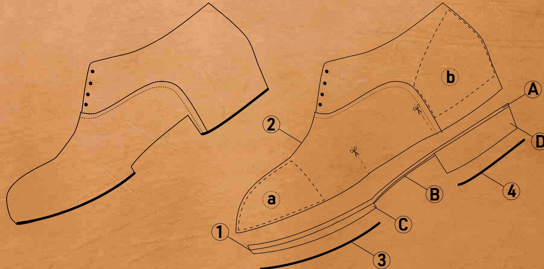
② **Uppers:** Cut and Sew the Uppers and reinforce eyelets and weak spots. Assemble with Leather Lining and start Lasting. During Lasting add Leather Toe Puff (a) and Heel Counter (b). After Determining the Uppers position, make an incision where Upper and the Waist of shoe meet. The Upper's Leather should cover the Shank Area. When lasting is completed add 2mm Rubber Midsole ③ and 6mm Rubber Heel ④ and fix with decorative nails
