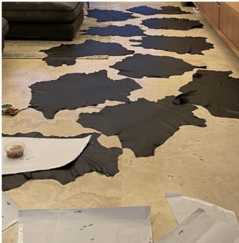
Pattern division according to leather hide sizes & alignment of style line continuity
