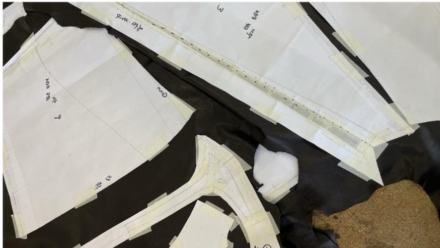
Pattern division according to leather hide sizes & alignment of style line continuity
