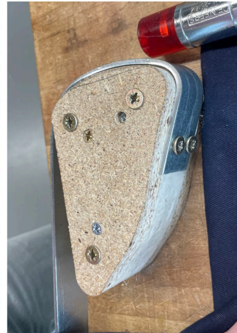
③ curving it cold by hand was easiest but had to drill the form into the table.
